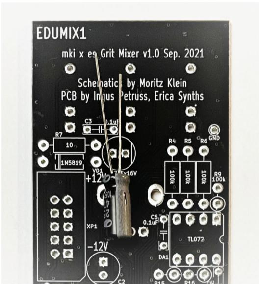
**Next, insert & solder the film- and electrolytic capacitors.** Electrolytic capacitors are bipolar, and you need to mind their orientation. The positive lead of each electrolytic capacitor is longer, and there's a minus stripe on the side of the capacitor's body to indicate the negative lead. On our PCBs, the positive pad for a capacitor has a square shape, and the negative lead should go into the pad next to the notch on the silkscreen.
