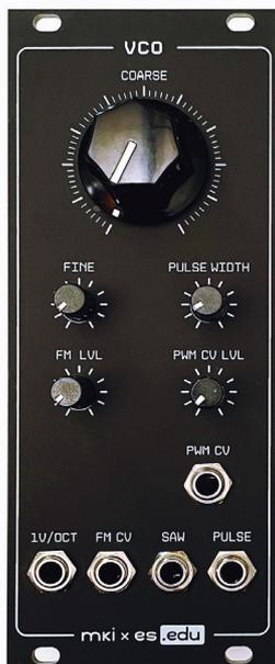
**Install the front panel** and fix it in place with the 5 hex nuts on the jack sockets and a washer plus hex nut on the top potentiometer. Fit the large knob on the bare potentiometer shaft and fix it in place with a small screwdriver. We are almost done
